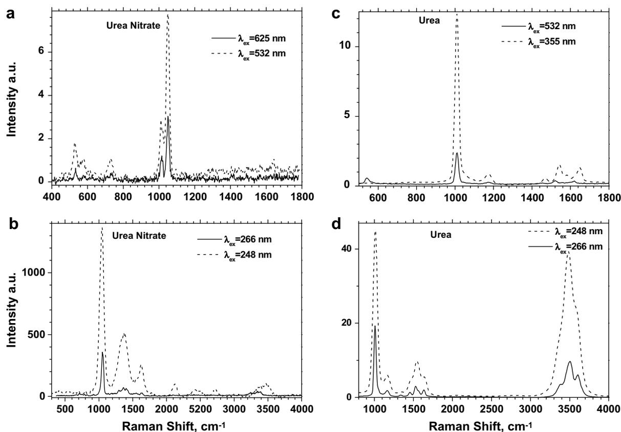
Fig. 4. Raman spectra of: Urea Nitrate (a,b); Urea (c,d).
