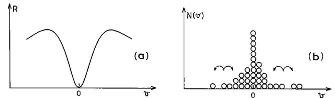
FIG. 5. Subrecoil laser cooling. (a) the random walk of the atom in velocity space is supposed to be characterized by a jump rate  $R$  which vanishes for  $v=0$ . (b) as a result of this inhomogeneous random walk, atoms which fall in a small interval around  $v=0$  remain trapped there for a long time, on the order of  $[R(v)]^{-1}$ , and accumulate.
