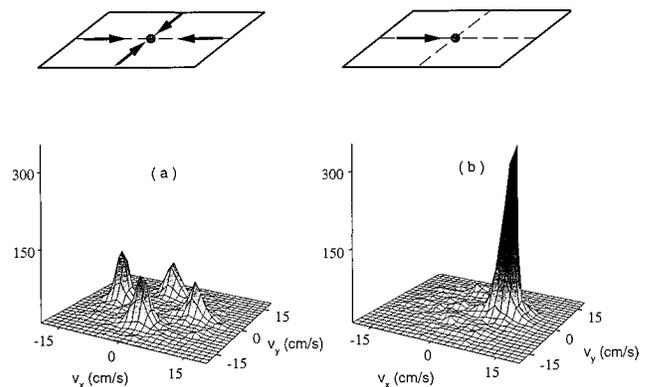
FIG. 9. Two-dimensional VSCPT experiment (from Kulin *et al.*, 1997). The experimental scheme is the same as in Fig. 7, but one uses now four VSCPT beams in a horizontal plane and atoms are pumped into a linear superposition of four different momentum states, giving rise to four peaks in the two-dimensional velocity distribution (a). When three of the four VSCPT laser beams are adiabatically switched off, the whole atomic population is transferred into a single wave packet (b).
