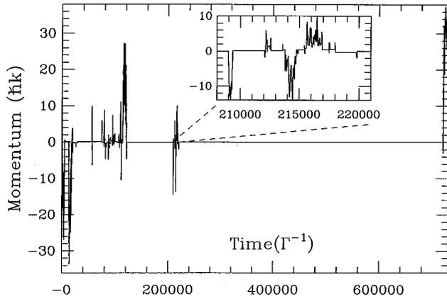
FIG. 10. Monte Carlo wave function simulation of one-dimensional VSCPT (from Bardou, Bouchaud *et al.*, 1994). Momentum  $p$  characterizing the cooled atoms vs time. Each vertical discontinuity corresponds to a spontaneous emission jump during which  $p$  changes in a random way. Between two successive jumps,  $p$  remains constant. The inset shows a zoomed part of the sequence.
