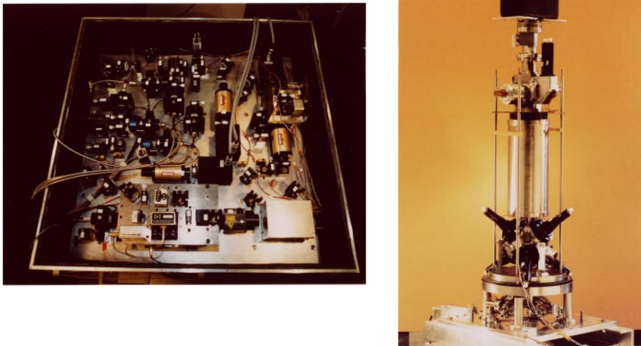
FIG. 11. (Color) The microgravity clock prototype. The left part is the 60 cm×60 cm×15 cm optical bench containing the diode laser sources and the various optical components. The right part is the clock itself (about one meter long) containing the optical molasses, the microwave cavity and the detection region.
