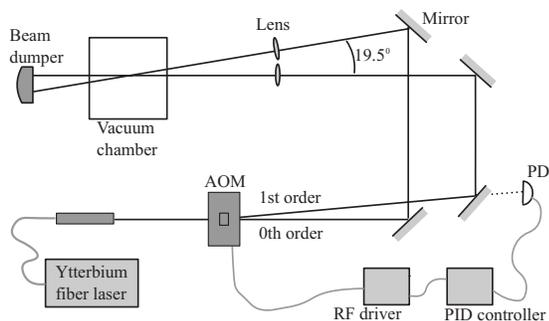
FIG. 1. A schematic representation of the optical-dipole trap experimental setup. The first-order diffraction beam is focused to a waist of  $31 \mu\text{m}$  and aligned to the MOT center. The zeroth-order beam is weakly focused to  $300 \mu\text{m}$ . It crosses the first-order beam at an angle of  $19.5^\circ$  and it only becomes important at the final stages of evaporation. AOM: acousto-optic modulator. PD: photodetector.
